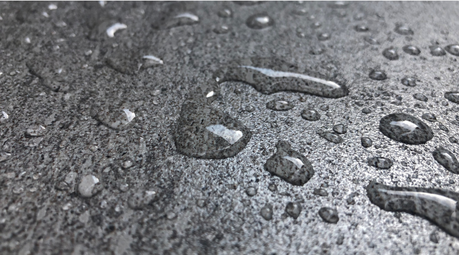
Swiss GriP applied to a dark ceramic tile, showing the "water-repellent" effect
